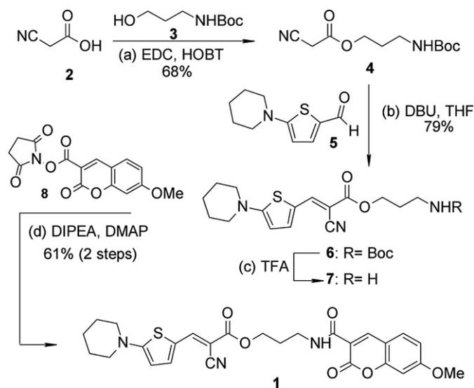
Fig. 1. Synthesis of the ratiometric molecular rotor **1**.
