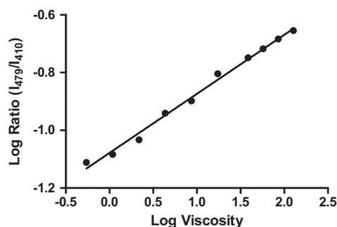
**Fig. 4.** Calculated emission intensity ratio versus viscosity for ratiometric dye **1**. Ratio  $I_{479}/I_{410}$  refers to the peak rotor emission divided by the reference emission for ratiometric dye **1** in ethylene glycol and glycerol. Both the viscosity and ratiometric intensity were log-transformed and then plotted. These values were taken from the reference excitation spectra in Fig. 2.
