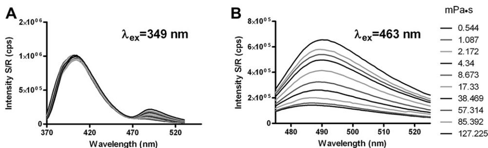
**Fig. 2.** Indirect excitation of the rotor through reference excitation (A) and direct rotor excitation (B) emission scans of ratiometric dye **1** in ethylene glycol and glycerol gradient. In the reference excitation graph, the low variability of the reference relative to the rotor emission ( $\approx 410$  nm) highlights the ratiometric properties. The rotor excitation graph confirms the viscosity sensitivity of the molecular rotor.
