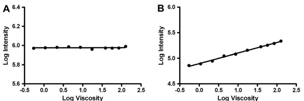
**Fig. 3.** Plot of ratiometric dye **1** peak emission from the single excitation measurement in Fig. 2. As expected, Fig. 3A exhibits no correlation between viscosity and the reference peak emission. Fig. 3B highlights the molecular rotor emission peak as a function of viscosity and confirms a significant correlation ( $R^2 = 0.9945$ ) with a slope of 0.21.
