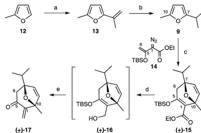
Scheme 4. Reagents and conditions: a) *n*BuLi (0.94 equiv), Et<sub>2</sub>O, –20°C, reflux; then –20°C, acetone (1.1 equiv), reflux; then Ac<sub>2</sub>O (1.5 equiv), KOAc (0.63 equiv), 110°C; b) Pd/C (catalytic), H<sub>2</sub> (1 bar), 1 h; c) [Rh<sub>2</sub>(Ooct)<sub>4</sub>] (2 mol%), hexanes, reflux, 95%; d) DIBAL-H (2.5 equiv), CH<sub>2</sub>Cl<sub>2</sub>, –78°C; e) BF<sub>3</sub>·Et<sub>2</sub>O (1.5 equiv), CH<sub>2</sub>Cl<sub>2</sub>, –30°C, 81%. DIBAL-H = diisobutylaluminum hydride.
