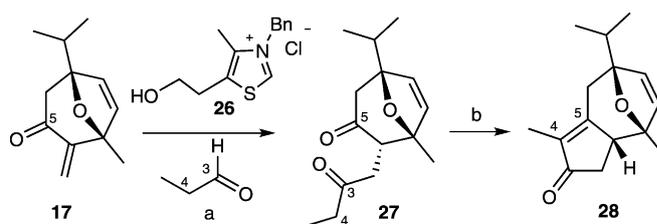
Scheme 7. Reagents and conditions: a) propanal (4 equiv), compound **26** (20 mol%),  $\text{Et}_3\text{N}$  (1.2 equiv),  $80^\circ\text{C}$ , 75%; b) KOH (5 equiv), EtOH, RT, 76%.
