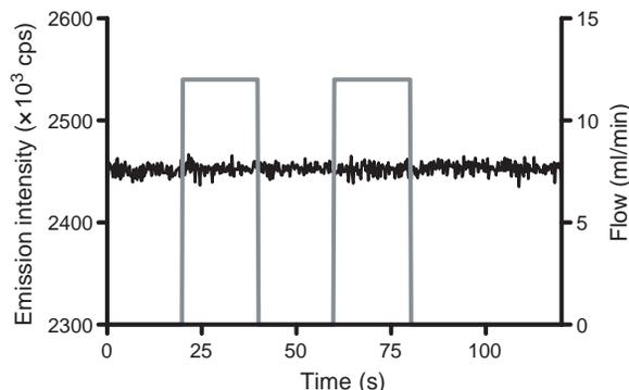
**Fig. 7.** Timecourse experiment using 10  $\mu\text{M}$  DCVJ in ethylene glycol. As opposed to both CCVJ and CCVJ-TEG, no changes in intensity were observed, in spite of relatively high flow rates.
