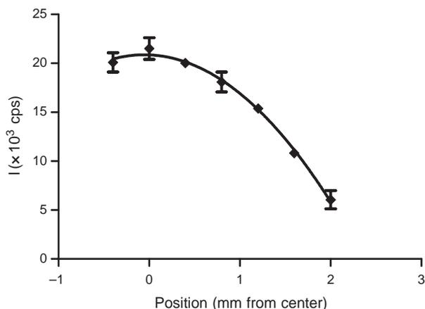
**Fig. 10.** Intensity increase caused by constant flow but with varying radial position of the fiber tip in a cylindrical tube. Shown is means  $\pm$  SD of three experiments. Maximum intensity increase was seen in the tube center, with a marked reduction towards the tube wall. A parabolic profile, following the flow velocity equation in a cylinder (Eq. 1), shows an excellent fit into the data.
