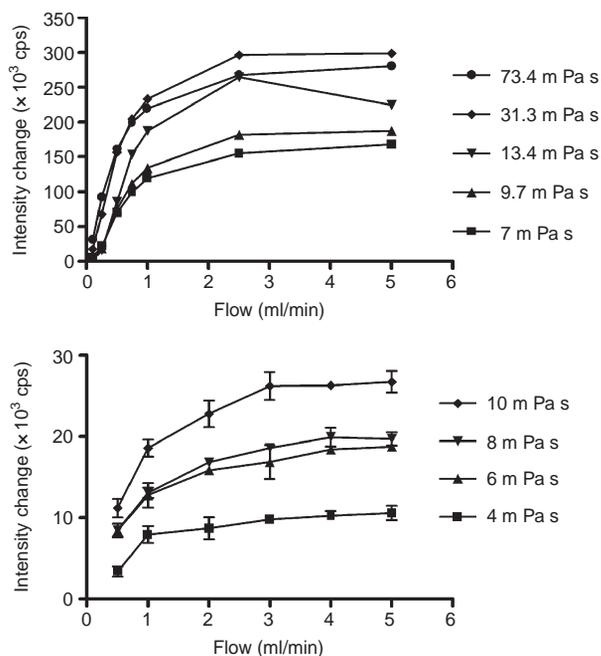
**Fig. 9.** Matrix experiment where intensity increase was observed at different flow rates in fluids of different viscosities (mixtures of ethylene glycol and glycerol). Shown are the dyes CCVJ (left) in a single experiment and CCVJ-TEG (right) as means and SD of four experiments. Intensity increase can be seen with both flow and viscosity, indicating that the effect is based on shear stress rather than shear rate.
