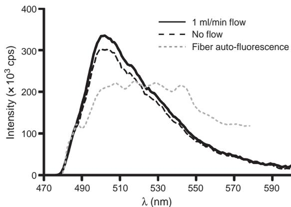
**Fig. 5.** Background-corrected fluorescence emission spectrum of 10  $\mu\text{M}$  CCVJ in ethylene glycol without flow and at 1 ml/min flow. Spectroscopy indicates that emission intensity increases with flow. No spectral shifts were observed. The background signal (fiber immersed in ethylene glycol without dye) that was subtracted from the dye spectra is shown as grey dotted line.
