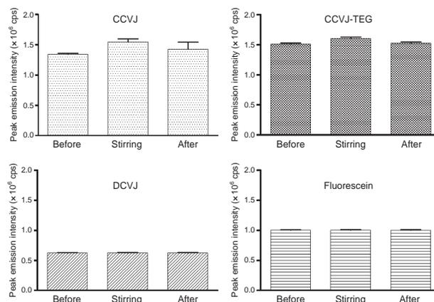
**Fig. 4.** 10  $\mu$ M CCVJ in ethylene glycol in a fluorometer cuvette before the stirrer was activated, during, and after stirring. Slow stirring increases both CCVJ and CCVJ-TEG intensity significantly (*t*-test,  $p < 0.05$ ) over unstirred control. Two control dyes, DCVJ and fluorescein do not show this increase (*t*-test, n.s.).
