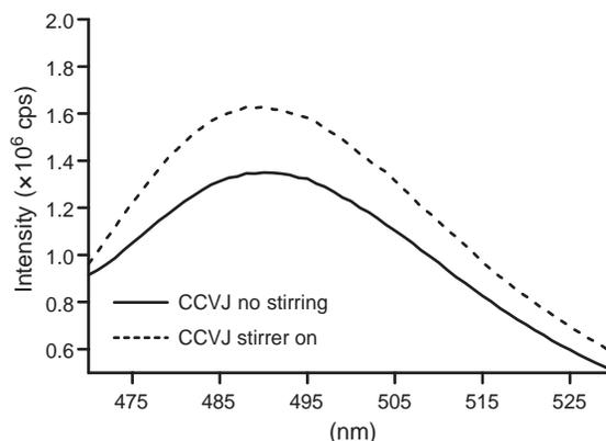
**Fig. 3.** Emission spectra of 10  $\mu$ M CCVJ in ethylene glycol, taken in a fluorometer cuvette with and without stirring.
