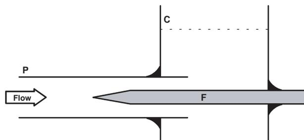
**Fig. 1.** Sketch of the fiberoptic shear apparatus. The optical fiber F with an etched tip was placed in the center of a glass pipette P. A small plastic container C served as fluid repository and also held the pipette and the fiber in position. The tip was inserted 20 mm upstream of the pipette end to keep it in an undisturbed flow region. Flow was applied to the far end of the pipette by means of a syringe pump.
