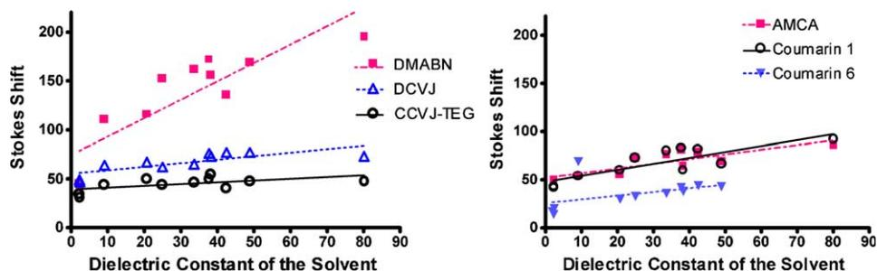
Fig. 5. Stokes shift of the different dyes in dependency of the dielectric constant of the solvents. DMABN shows the highest increase of the Stokes shift (slope  $m = 1.9$ ,  $r^2 = 0.75$ ). The slope is markedly lower with the molecular rotors (DCVJ:  $m = 0.36$ ,  $r^2 = 0.6$ , CCVJ-TEG:  $m = 0.18$ ,  $r^2 = 0.35$ ) and the Coumarins (AMCA:  $m = 0.49$ ,  $r^2 = 0.73$ ; Coumarin 1:  $m = 0.62$ ,  $r^2 = 0.71$ ; Coumarin 6:  $m = 0.39$ ,  $r^2 = 0.2$ ).
