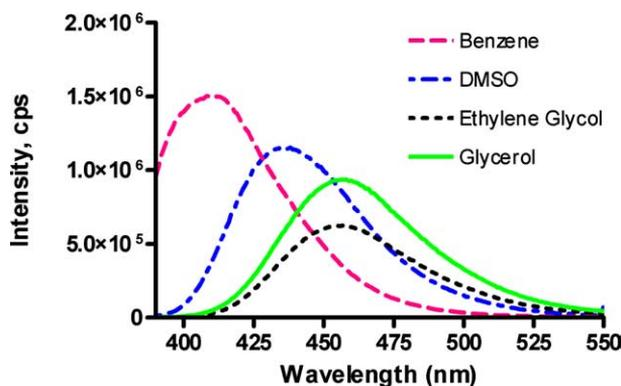
Fig. 3. Emission spectra of Coumarin 1 in selected solvents. No secondary emission peak was seen, but the emission spectra markedly shifted to the red in more polar solvents.
