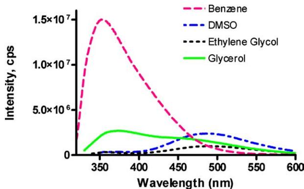
Fig. 2. Emission spectra of DMABN in selected solvents. DMABN shows the highest emission intensity in nonpolar solvents (benzene) and exhibits a secondary, red-shifted emission peak in polar solvents (e.g., DMSO and ethylene glycol). This secondary peak originates from deexcitation from the TICT state. In glycerol, the higher viscosity partially inhibits TICT formation, and deexcitation takes place predominantly from the LE state.
