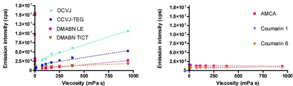
Fig. 8. Dependency of the peak emission intensity on the viscosity of the solvent. The Coumarin dyes exhibit only a very weak dependency of the peak emission on the viscosity. The molecular rotors and, to a lesser extent, DMABN, show increased peak emission with solvent viscosity. However, nonpolar solvents with low-viscosity increase DMABN emission from the LE state more than highly viscous solvents.
