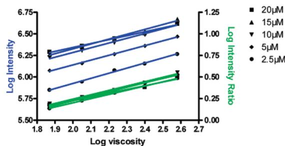
**Figure 4.** Reduction in the influence of dye concentration using ratiometric measurements. Blue lines correspond to CMAM emission in mixtures of ethylene glycol and glycerol (dye concentration 2.5–20  $\mu\text{M}$ ). Green lines correspond to the CMAM emission divided by the MCCA emission. Ratiometric measurement dramatically reduces variations between samples despite the high range of concentrations used.
