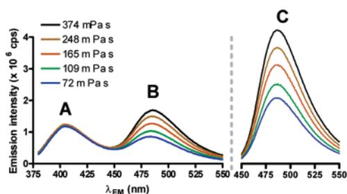
**Figure 3.** Emission spectra of probe **4** in mixtures of ethylene glycol and glycerol. Peaks A, B, and C correspond to MCCA (reference), RET, and CMAM emissions, respectively. Peaks A and B were acquired at  $\lambda_{\text{ex}} = 360$  nm, while peak C was acquired at  $\lambda_{\text{ex}} = 444$  nm. Only peaks B and C are viscosity-dependent.
