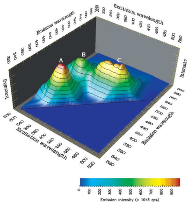
**Figure 2.** Fluorescent fingerprint of dye **4**. Peak A ( $\lambda_{\text{ex}} = 360$  nm and  $\lambda_{\text{em}} = 402$  nm) corresponds to the donor fluorescence peak (MCCA). Peak B ( $\lambda_{\text{ex}} = 349$  nm and  $\lambda_{\text{em}} = 481$  nm) corresponds to the RET, while peak C ( $\lambda_{\text{ex}} = 449$  nm and  $\lambda_{\text{em}} = 486$  nm) is emitted by CMAM.
