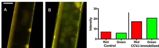
Fig. 2. (Color online) Epifluorescent image of the fiber tip sections where the cladding was removed. Both fibers were illuminated at the distal end with a 440 nm laser. Image A shows a fiber without any immobilized dye (control). The emitted light is caused by fiber autofluorescence. Image B shows a fiber with immobilized CCVJ (5a). Stronger green emission intensity, on average 20% higher than that of the control fiber, is clearly visible. The scale bar is 150  $\mu\text{m}$ .
