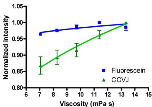
Fig. 4. (Color online) Viscosity-intensity relationship of immobilized CCVJ (**5a**) and FRS (**5b**) under internal illumination of the tip. The error bars indicate standard deviation for  $n=4$  independent experiments.
