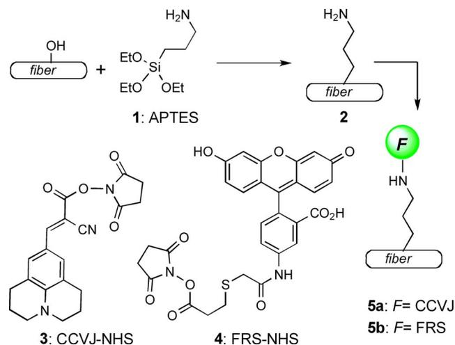
Fig. 1. (Color online) Functionalization of a fiber-optic tip with either CCVJ or fluorescein (FRS).
