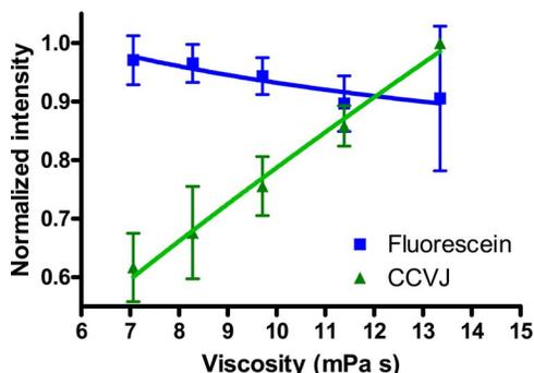
Fig. 5. (Color online) Viscosity-intensity relationship of fiber immobilized CCVJ (**5a**) and FRS (**5b**) under external laser illumination of the tip. The error bars indicate a standard deviation for  $n=4$  independent experiments.
