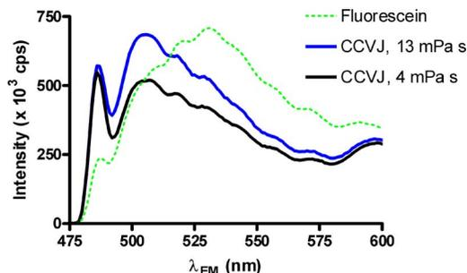
Fig. 3. (Color online) Emission spectra of immobilized CCVJ (5a) and FRS (5b) when excited through the fiber at 440 nm. CCVJ emission intensity increases in fluids of higher viscosity.
